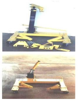
Note: When the Hydraulic Jack (Attached to Book Extension) is lowered down, the HEIGHT of the hoist is only 4"!!!!!!!!!
